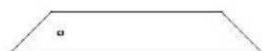
E6 | CALE DE PLATEFORME - W4L15942 (8) | 1 7/16 po x 3 3/8 po x 20 po (36 x 86 x 508)
