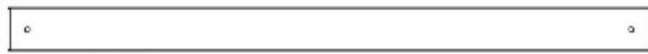
M10 | RAIL MURAL DU PAVILLON - W4L04614 (1) 5/8 po x 3 3/8 po x 50 1/4 po (16 x 86 x 1277)
