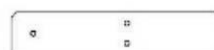
H24 | SUPPORT TABLE DE PIQUE-NIQUE - W4L04601 (1) 1 po x 3 3/8 po x 16 1/2 po (24 x 86 x 418)
