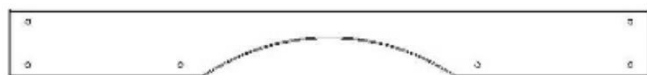
K5 | RAIL MURAL DU PAVILLON - W4L04626 (1) | 5/8 po x 5 1/4 po x 50 1/4 po (16 x 134 x 1277)
