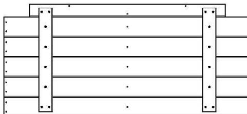
FP1 | PANEL DEL PISO - W2A02865 (x2) | 1 1/4"x19 1/8"x41 7/8" (36x485x1064)
